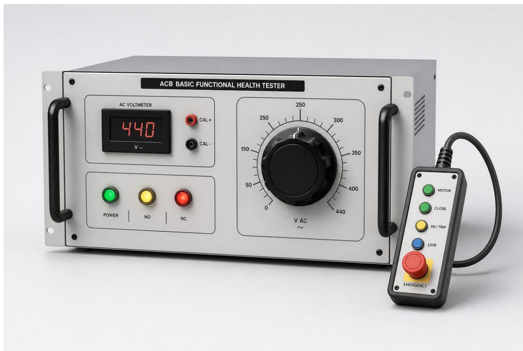
Figure 1: Illustrative image of ACB Basic Functional Health Tester with pendent
